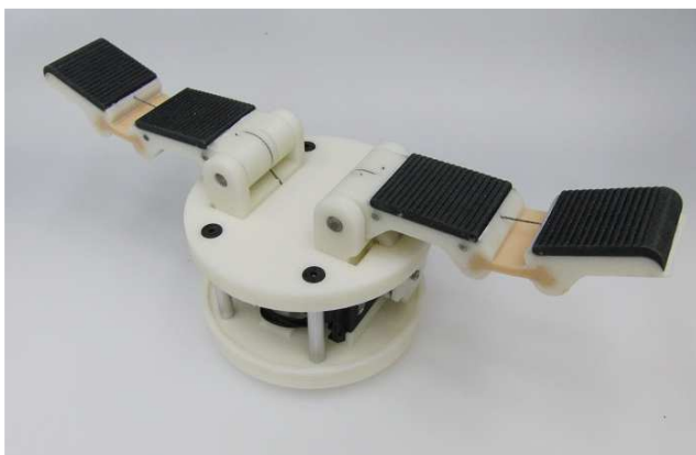
Fig 3. Model T42, more dexterous than the Model T, while maintaining benefits of adaptability through underactuated fingers
