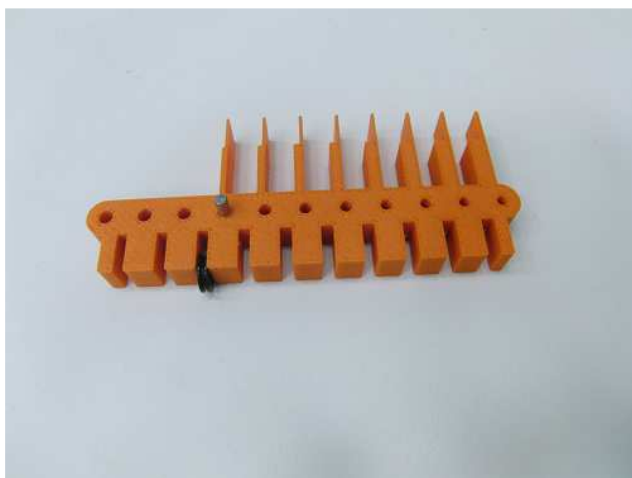
Fig 7 – example calibration piece that may help with setting the appropriate printing parameters
