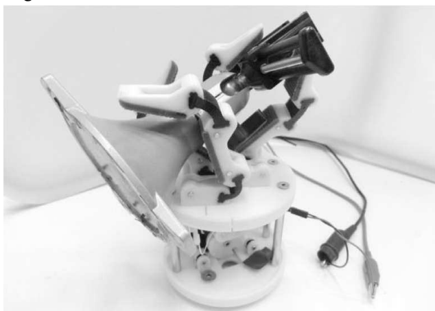
Fig 5. Example case of the passive adaptability made possibly by compliant flexure joints.
